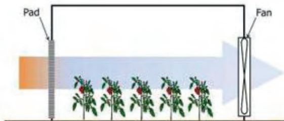
Image of the Pad and Fan
