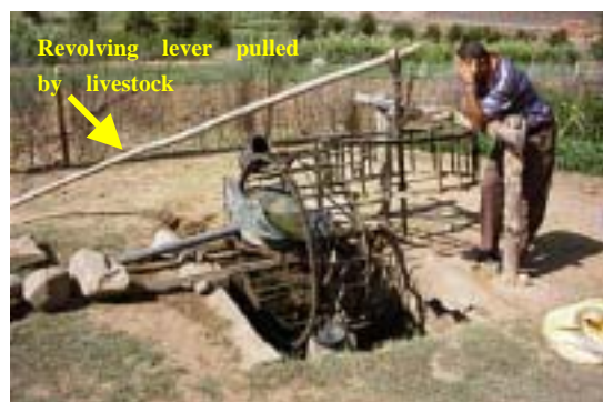
Photo 2: Shallow well using livestock power
